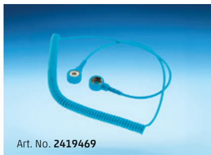
Designation Spiral cable extremely flexible 2.4 m x 2 x 1 MOhm safety resistance Earth connection: 10 mm push-button
