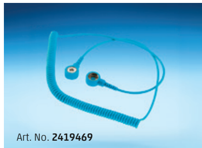
Art. No. 2419469 Designation Spiral cable extremely flexible 2.4 m x 2 x 1 MOhm safety resistance Earth connection: 10 mm push-button
